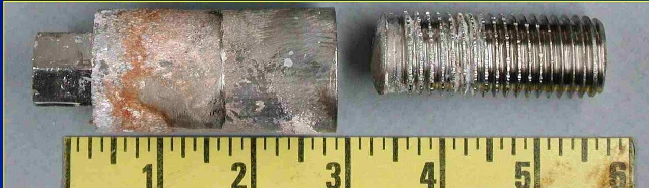
*Fatigue failure in a bolt*
