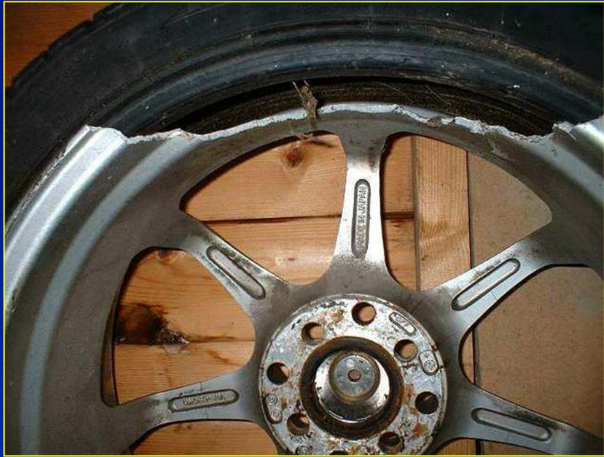
*Fatigue failure occurs at the outer rim of the wheel*
