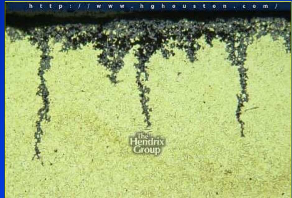
**Corrosion fatigue of brass**
