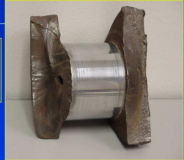
*Failure of crankshaft journal*
