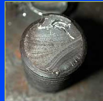
*Fatigue failure of a bolt*
