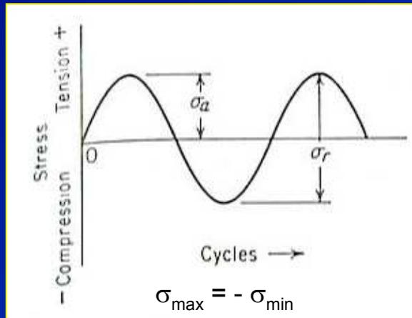
(a) Completely reversed cycle of stress (sinusoidal)
